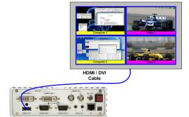
3. Connect one end of the DVI / VGA / YPbPr signal cable (a VGA-to-DVI converter may be required) to the DVI-I IN COMPUTER 1 connector on the rear panel. Connect the other end to the first computer system's DVI / VGA port.
