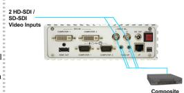
Connect the Ethernet cable from the **IP** port on the Sequoia's rear panel to the router. Connect one Ethernet cable from the router to the first computer and another Ethernet cable from the
