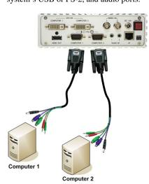
IMPORTANT: You are highly recommended to use the USB 4. connection when available instead of the PS-2 connection. In case no USB connection is available and you have to use the PS-2 connection, make sure to first turn on power to your Sequoia (refer to a later step), then turn on power to your computer system afterwards.
