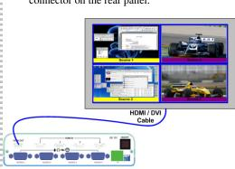
3. Connect one end of the HDMI / DVI signal cable (a DVI-to-HDMI converter may be required) cable to the **HDMI IN 1** connector on the rear panel. Connect the other end to the first computer system's HDMI / DVI port. Connect another HDMI / DVI signal cable to the **HDMI IN 2** connector on the rear panel and the other end to the second computer system's HDMI / DVI port. Do the same for the third and fourth computer.
