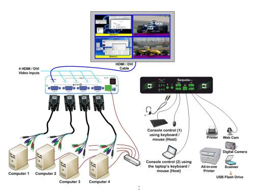
. Connect one end of the Sequoia all-in-one cable to the **SOURCE 1** connector on the rear panel. Connect the other end to the first computer system's USB or PS-2, and audio ports by matching the colors of the respective connector. Connect another Sequoia all-in-one cable to the **SOURCE 2 / 3 / 4** connectors on the rear panel and the other end to the second / third / fourth computer system's USB or PS-2, and audio ports.
