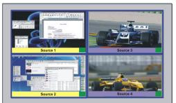
to the active window. To enable audio output would correspond to the active window. To enable audio output other than the active window, disable the item Audio Output from Active Window (remove checkmark) under Settings -> System Parameter -> Sequoia Properties in the Galaxy program (refer to chapter 3 of the User Manual for details).
